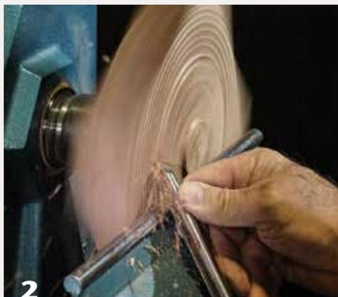
2 Turning the underside of the piece by rolling the tool into the wood.
