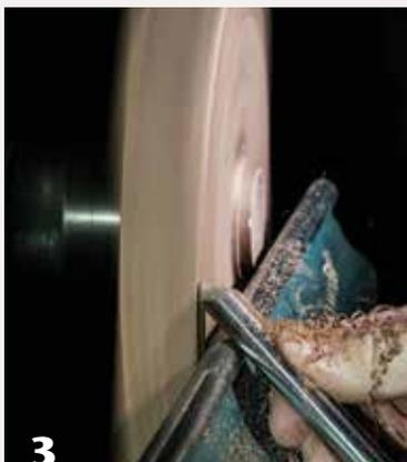
3 Final cuts toward the center with the bevel lightly in contact with the wood.
