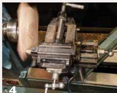
4 Using the cross-slide vise to make a perfectly flat cut.
