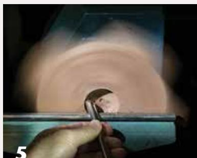
5 Turning out the center of the sphere was straightforward, like hollowing a bowl.
