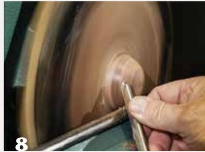
The jig for mounting the piece to finish-turn the bottom of the sphere. A jam fit and duct tape hold the piece firmly in place.
