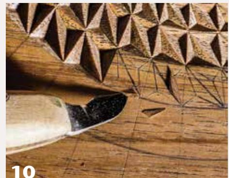
Zina's drawn design becomes tangible in wood. Her first two cuts, rolling the tool tip forward into the wood, produce a chip that is released with a third cut.
