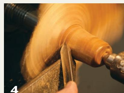
4 Turning a spigot for remounting in a chuck
