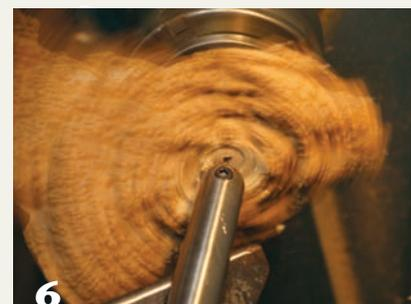
6 Roughing a flat spot in the center where a recess will be drilled
