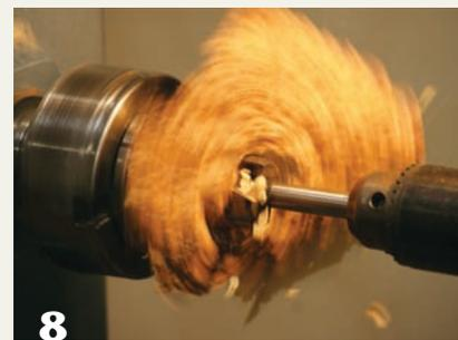
8 Drilling the recess using the saw-tooth drill bit
